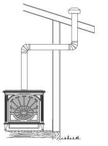
Figure 24 - Venting Through a Side Wall
